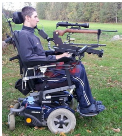
Richten met kin-besturing Fabrikant: Adaptive Shooting System LLC
